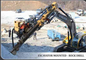
EXCAVATOR MOUNTED - ROCK DRILL
